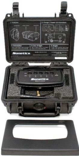
Fig. 1: Removal of faceplate.
