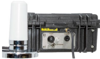
Fig. 3: External antenna connection.
